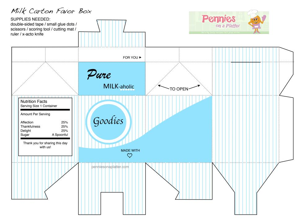
INSTRUCTIONS: Print the favor box onto white cardstock, and cut out along the solid lines with scissors or an x-acto knife. Fold along the dotted lines, using a scoring tool and a ruler to score before folding for easier assembly. Use double-sided tape or glue dots to attach the small side flaps to the "nutrition facts" side of the box. Finish assembling, add your treats, and slide the flap closure into the slot to finish.
